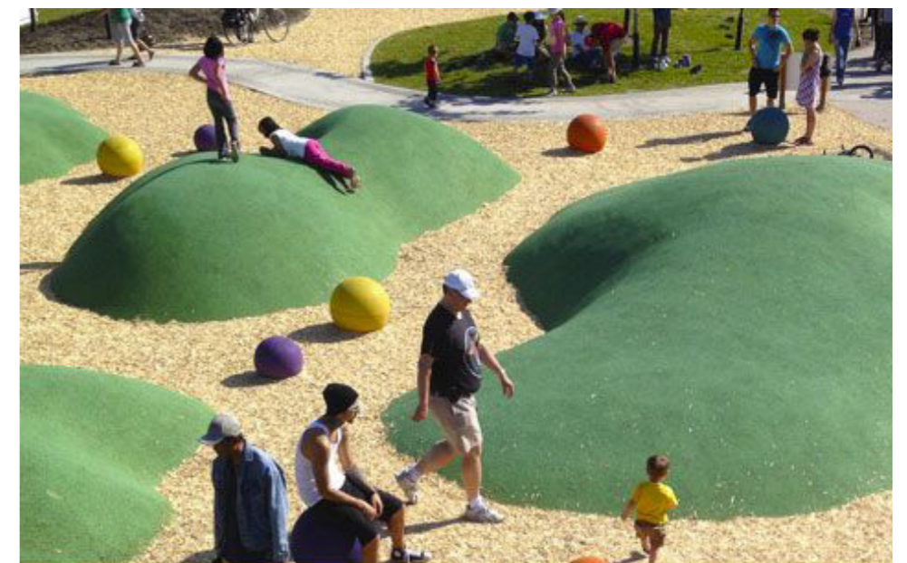
Wet pour safety surfacing mounds and for safety surfacing to fitness equipment
